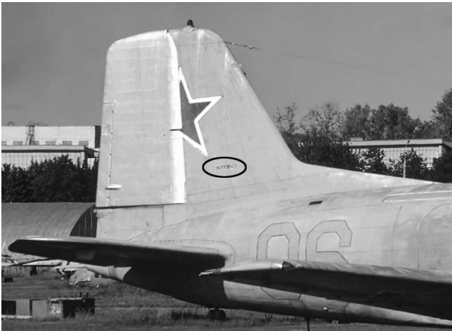
With (Soviet) military aircraft the construction number was in most cases painted on the tail. With some aircraft from the Khodynka productions and all aircraft from the Dresden production the construction number plate is to be found on the left hand side on the nose.
