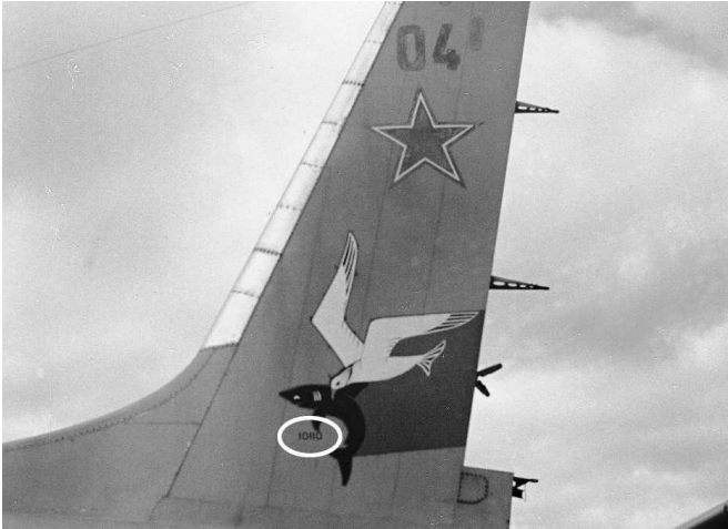
The Il-18 construction number is often painted on the tail and also to be noted on the forward underside of the wing, close to the fuselage.
