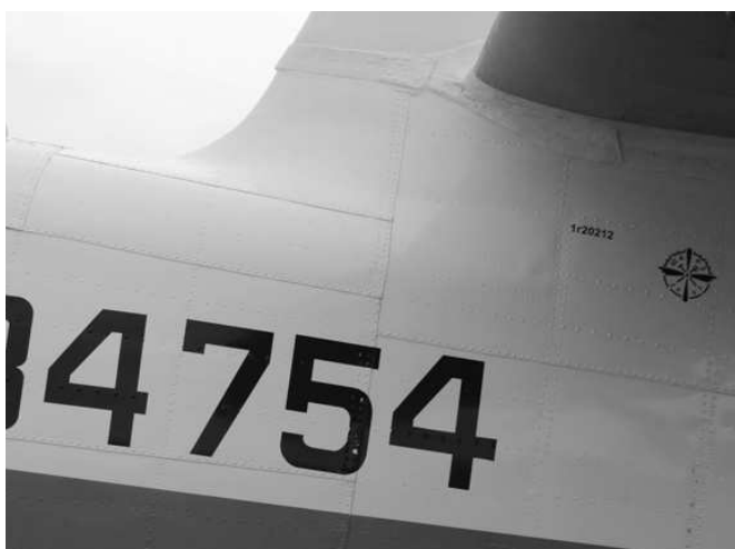
The construction number is normally painted under the horizontal stabilizer on the left-hand side. In rare cases (see photo above right) it is painted on the right-hand side.
