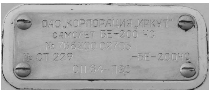
The construction number is found etched on a plate riveted to port side of rear fuselage below the waterline.
