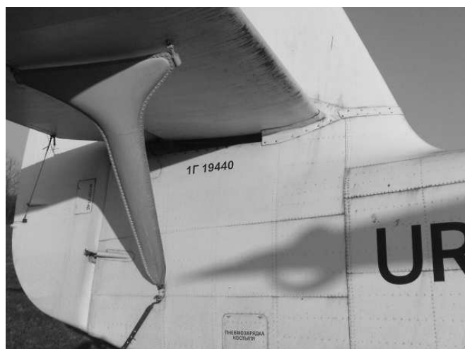
The construction number is normally painted under the horizontal stabilizer on the left-hand side. In rare cases (see photo above right) it is painted on the right-hand side.
