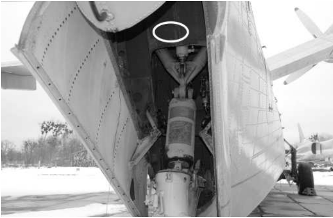
The Be-12 construction number plate is attached inside the tail wheel bay.
