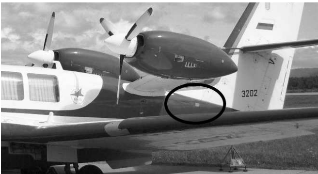
The construction number plate is on the left rear side of the fuselage below the rear end of the left engine.
