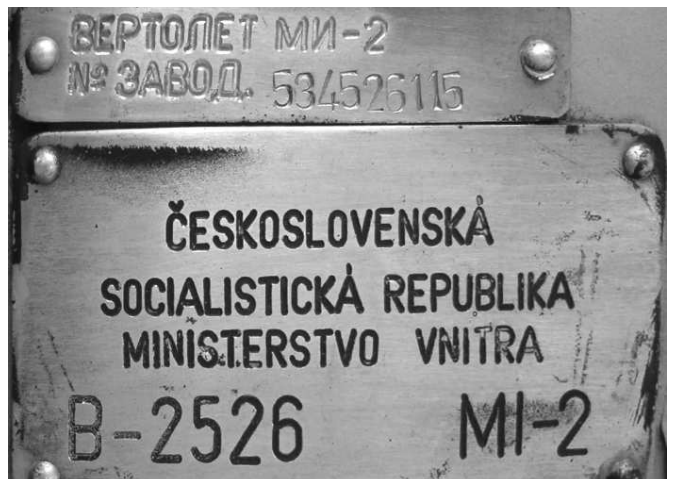
The construction number is normally painted on both sides of the tail boom. Preferably the plate has to be checked and this is to be found on the right side of the cockpit instrument panel and is easily readable from the outside.
