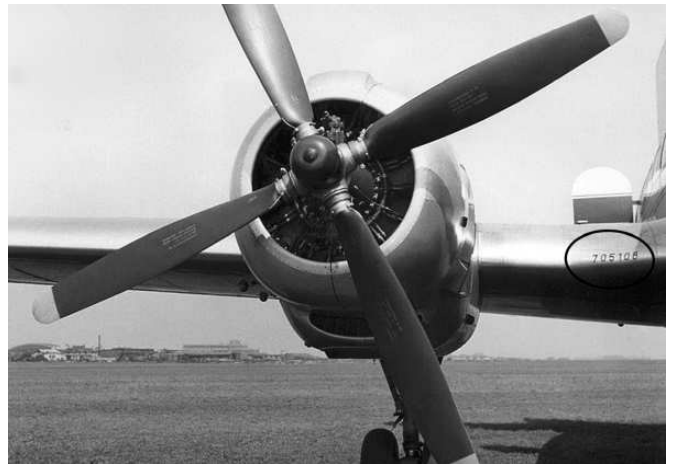
In some cases with both Il-12 and Il-14 the construction number was painted on the leading edge of the wing(s).
