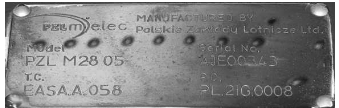
The construction number is often painted on the inside of both vertical stabilizers. The construction number plate is found under the horizontal tailplane on the left side.
