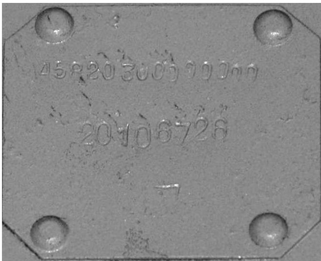
The construction number is painted in the bomb bay, visible when looking to the rear. It can also be found on the rear wall of the nose-wheel bay. Sometimes painted on and sometimes on a tiny plate (with the drawing number starting with 145 in the upper line and the construction number on the lower line). Apart from that, the construction number can be found on the plate of the nose-wheel strut (in the right upper corner of the plate).
