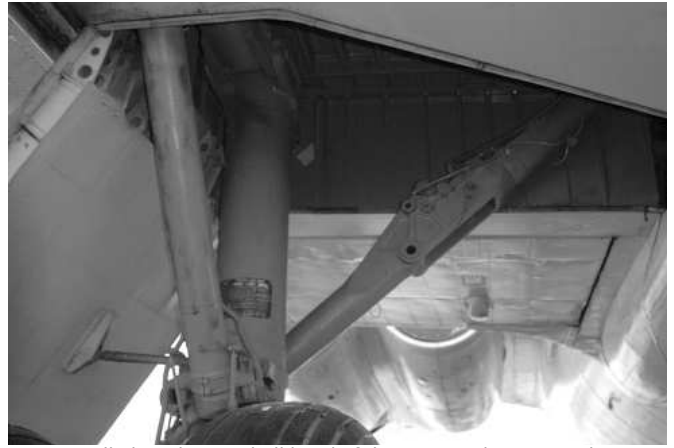
If access to the log book is not possible the Il-62 construction number can be seen stencilled on the rear bulkhead of the main undercarriage housing. The manufacturer's plate is to be found on the right main undercarriage.
