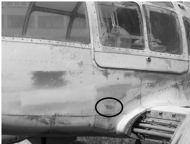
The construction plate is at the left side of the lower fuselage just in front of the wing root.
