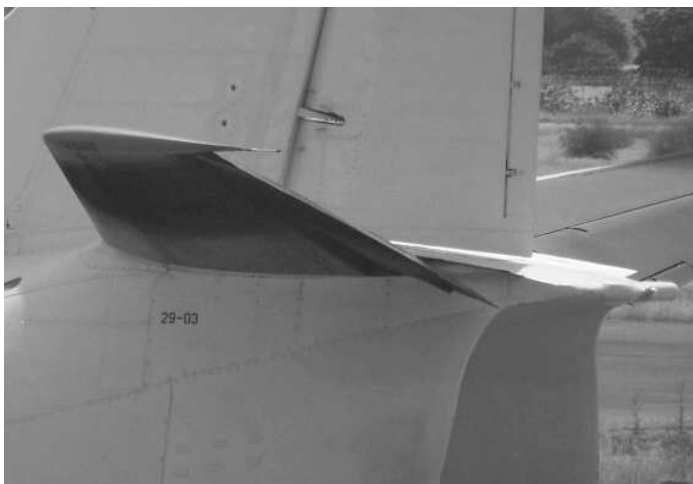
The construction number is normally stencilled under the horizontal stabilizer on the left side of the aircraft. In, at least, a Libyan An-32 the construction number plate was found in the rear cargo bay above the rear-most window on the left hand side at about eye-level.
