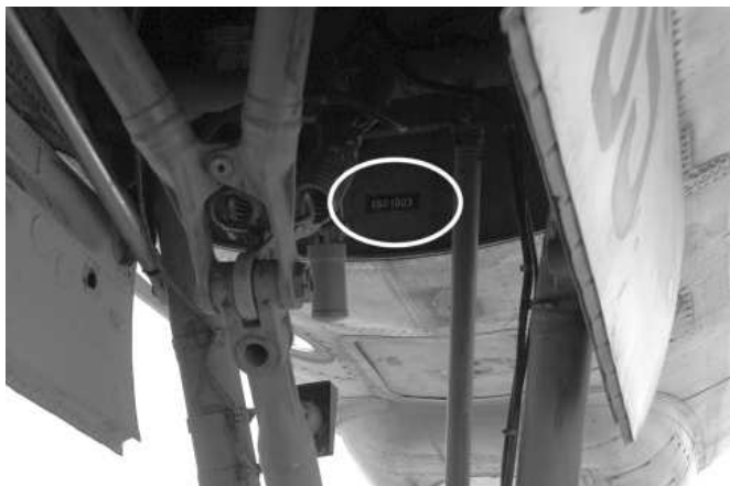
The construction number (or just its last five digits) is normally found in the nose wheel bay.
